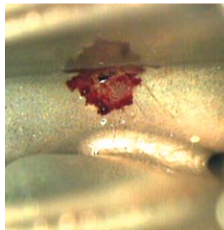
Figure 8.30 (b) Pitting corrosion in stainless steel 316.
