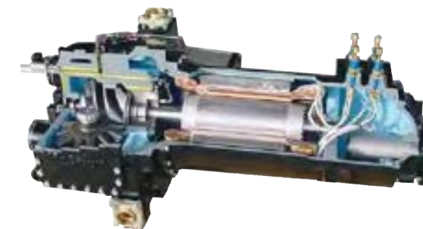
Figure 3.3 Single-screw compressor (Courtesy of McQuay International)
